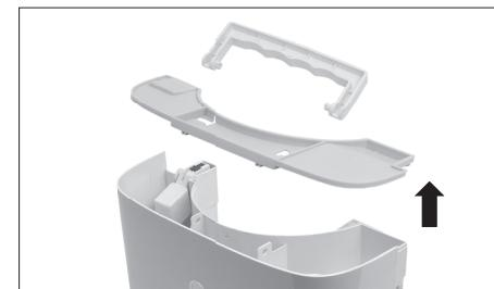
Dismount the water tank for cleaning and remount it in the reverse way before reinstalling it to the appliance
