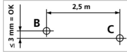
2.5 m to the right and mark point C. Check whether the horizontal line from point C is level with point B to within  $\pm 3$  mm. Repeat the process by turning the laser to the left.
