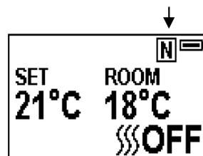
**NOTE: It is normal for the fan heater to stop running for periods of time. This happens because the room temperature is at or above the temperature set on the remote control. The heater indicator will be turned off after 10s if you have the flame ON. The heater indicator will stay ON if you use the heating function only.**
