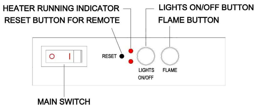
**NOTE:** The manual button controls basic functions, not a full range of controls. Use the remote hand set to carry out all functions.
