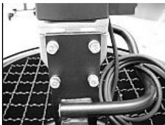
Fix the tool tightly to the stand by means of the 4 Allen screws M8 x 20 and the appropriate locking rings.
