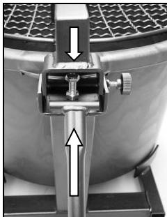
Fix the protective grid on the bucket and place the draw bar.
