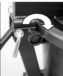
Insert the motor head with the stirrer basket into the bucket and lock it by turning the knurled screw in the direction of the arrow.
